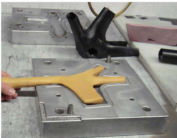
Stoner G471(XK-22) allows part to fall off the crushed mold.
